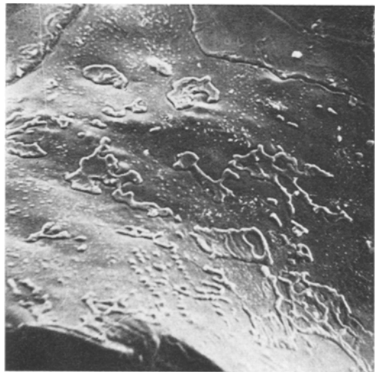
Figure 10 As fig. 4, showing that the form and shape of the "dark spots" closely resembles the characteristics of liquid droplets which have solidified on a metal surface ( \times 720 ).
